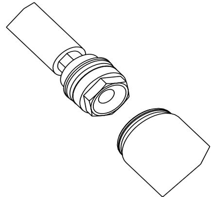
11. Install cylinder/shaft assembly into P/N 18227-00 pump Head, careful not to cut O-Ring for pump P/N 21835-00.
