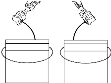
2. Flush system side to be rebuilt with suitable solvent.
