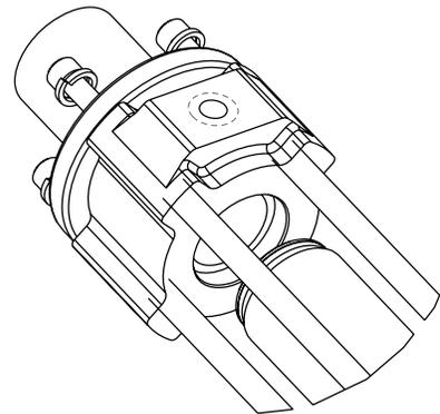
6. Remove Cup Adapter, P/N 21440-00 from Pump Head, P/N 18227-00.
