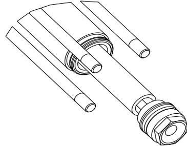
5. Remove cylinder, P/N 18219-00 from Pump Head, P/N 18227-00.
