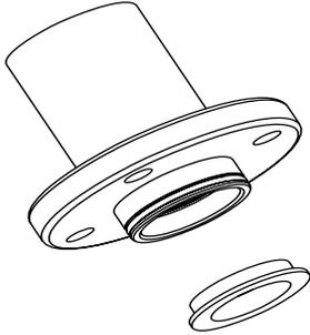
6. Place P/N 21595-00 Seal and P/N FS-110 guide on P/N 21597-00. The lips of the Seal will face away from P/N FS-110.
