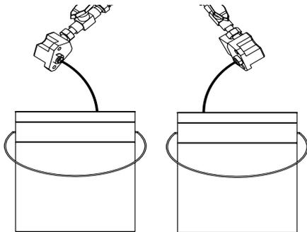
6. Close both side blocks simultaneously and wipe off residue from the side block seals. Regrease and attach both blocks to the gun.
