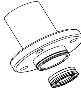
4. Lubricate and install O-Ring, P/N 13867-43 on bottom groove.
