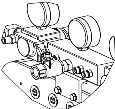
9. Generously coat the exposed transfer pump shafts with lithium grease.
