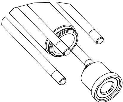
4. Using a rubber mallet, tap shaft out through the bottom of the cylinder, P/N 18219-00.
