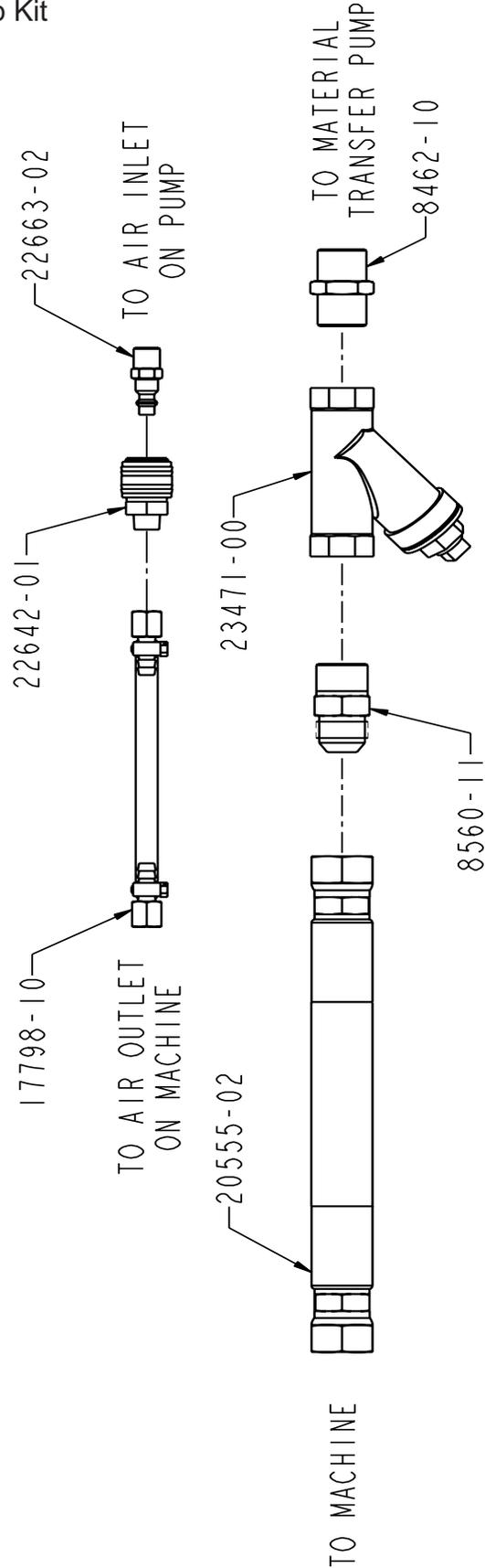
**Note:** The transfer kit attaches the same way for both ISO & POLY side. Use teflon tape on NPT threads.
