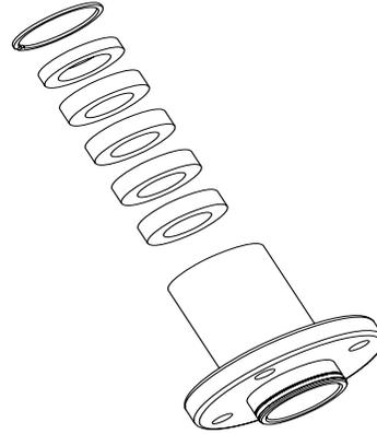
3. On bottom side of P/N 21440-00 install P/N 21595-00 so that the lip faces out
